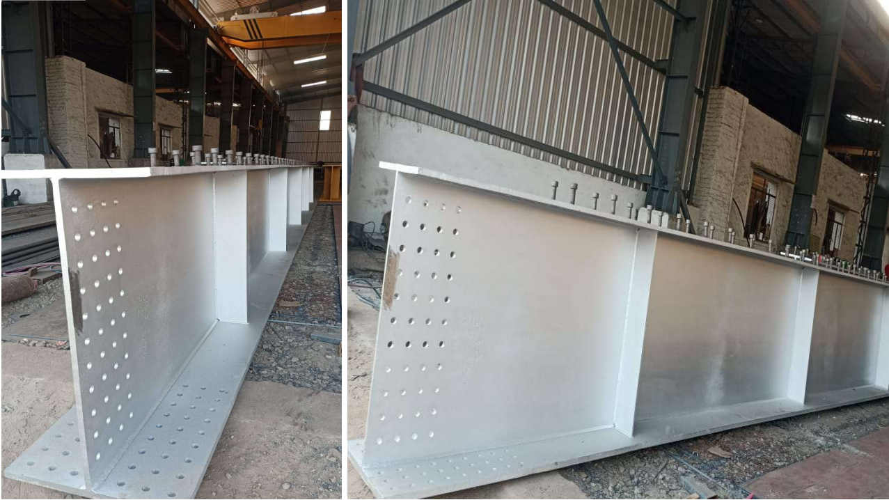
FOB GIRDER WITH STUD - 32+28M SPAN
